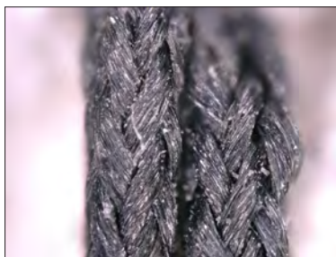
Fig. 13a: Black braided silk sutures magnified 200-fold with Keyence VHX-5000 microscope shows the texture of wax and silicone. Image: Nicole Ong Yii Mei
