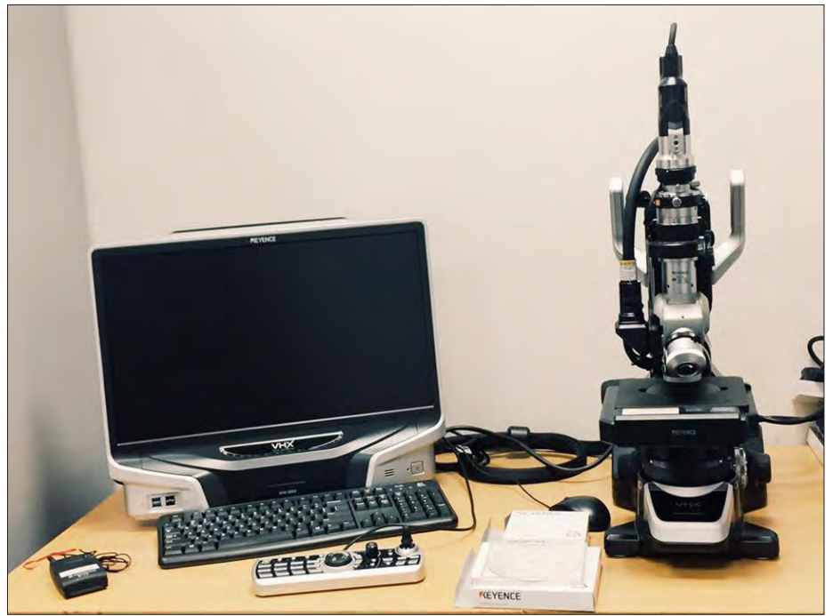
Fig. 11a: Keyence VHX-5000 microscope used to examine silk textile samples up to 2000x magnification. Image: Nicole Ong Yii Mei
